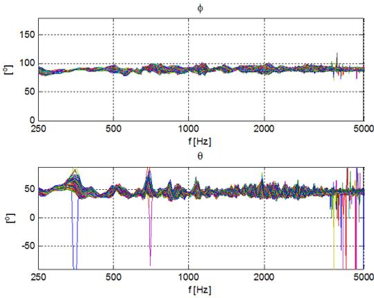
**Figure 6:** Angles determined with the non-linear LSPW-method for  $45^\circ$  incidence.
