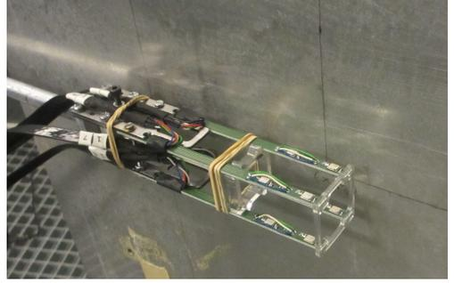
**Figure 3:** 3D sound intensity probe in front of a plate.
