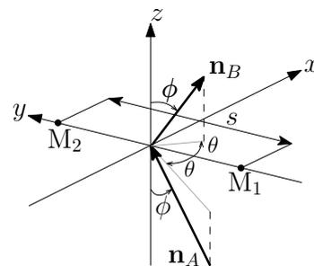
**Figure 2:** Direction convention in 3 dimensions.  $M_1$  and  $M_2$  indicate the positions of microphone 1 and 2.
