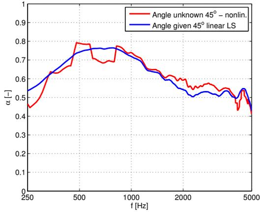
**Figure 5:** Area-averaged sound absorption coefficient for  $45^\circ$  incidence obtained with the linear least-squares and the non-linear Newton-Raphson solving procedure.
