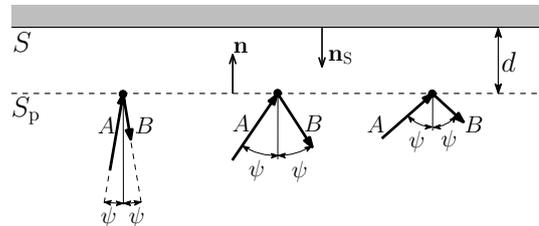
**Figure 1:** Approximation of an acoustic field locally by one incident ( $A$ ) and one reflected wave ( $B$ ).
