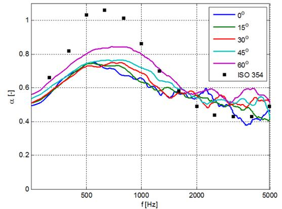
**Figure 4:** Area-averaged sound absorption coefficient for different angles of incidence obtained with the LSPW-method.
