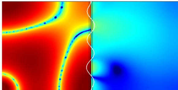
Figure 1: Sound pressure level distribution of the reference example; a sending room (left), an aluminium partition and an anechoic receiving room (right).
