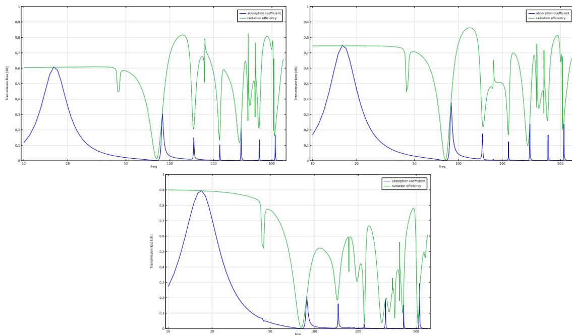
Figure 8: Absorption coefficient (blue line) and radiation efficiency (green line) according based on the LPW method for the anechoic receiving room (top left), rigid floor (top right), rigid floor and rigid right wall (bottom).
