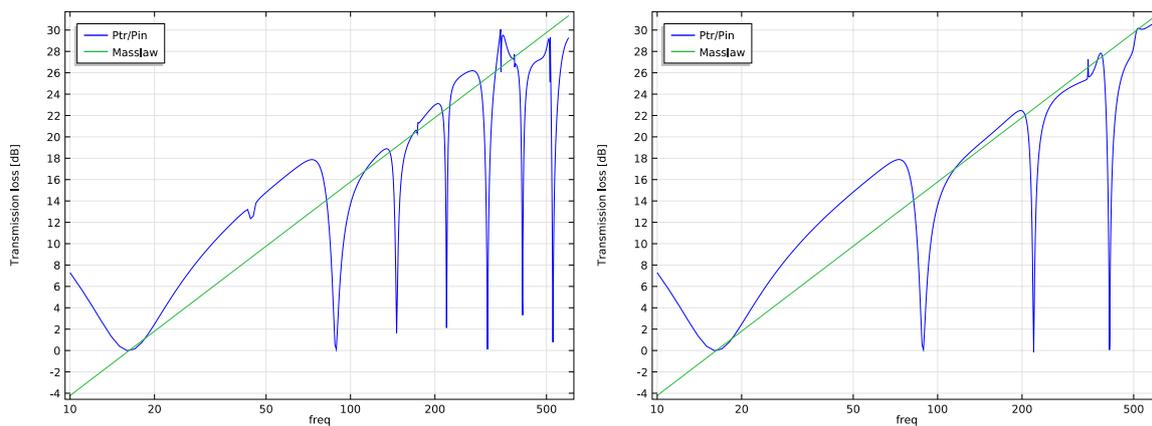
Figure 5: Transmission loss according to LPW (blue line) and the mass law (green line) for the reference example (left) and the example of a changed source position (right).
