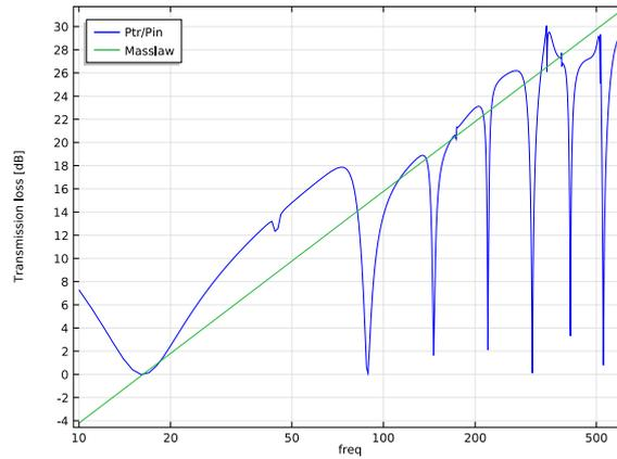
Figure 2: Transmission loss according to LPW for the reference example (blue line) and the mass law (green line). The point source is situated in the bottom-left corner in the sending room.
