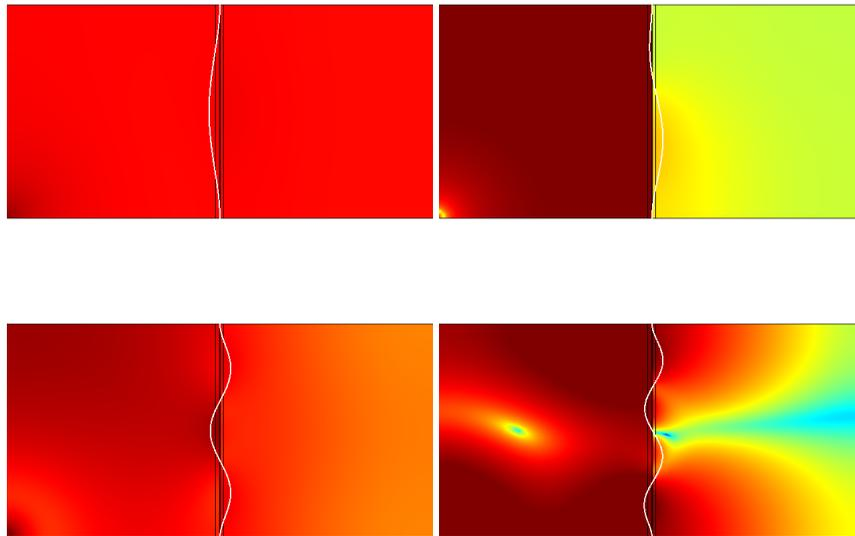
Figure 3: SPL for the reference example at 16 Hz (top, left), 44 Hz (top, right), 89 Hz (bottom, left) and 146 Hz (bottom, right). The point source is situated in the bottom-left corner of the sending room.
