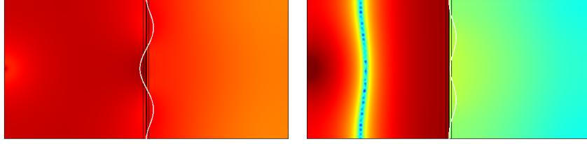
Figure 6: SPL at 89 Hz (left) and 146 Hz (right). As opposed to the reference example, the point source is located in the center of the left wall.
